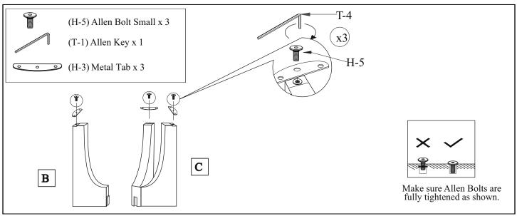
Align the holes on Metal Tab (H-3) with the pre threaded holes provided onto the top of Leg (B) & Twin Leg (C) as illustrated. Secure connection using Allen Bolt Small (H-5). And tighten it with Allen Key (T-1). Do not overtighten.
