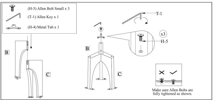
Position Twin Leg (C) upside down onto a padded, non-marring surface. While holding steady, engage the wooden extension on Leg (B) with the slot in Twin Leg (C) and slide down as illustrated. Once engaged, align the holes in the Metal Tab Y (H-4) with the pre threaded holes on the bottom of the Leg (B) and Twin Leg (C). Loosely secure the connection with Allen Bolts Small (H-5) using the provided Allen Key (T-1). DO NOT yet fully tighten.
