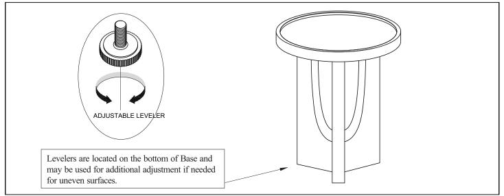
Using a second person to assist you, carefully turn the assembly upright. Assembly is now complete and the product is ready for use. Adjustable levelers are located on the bottom of each leg and may be adjusted by turning outwards, counter-clockwise to help account for uneven surfaces. NOTE: Hardware may loosen over time. Periodically check that all connections remain tight and adjust as needed.
