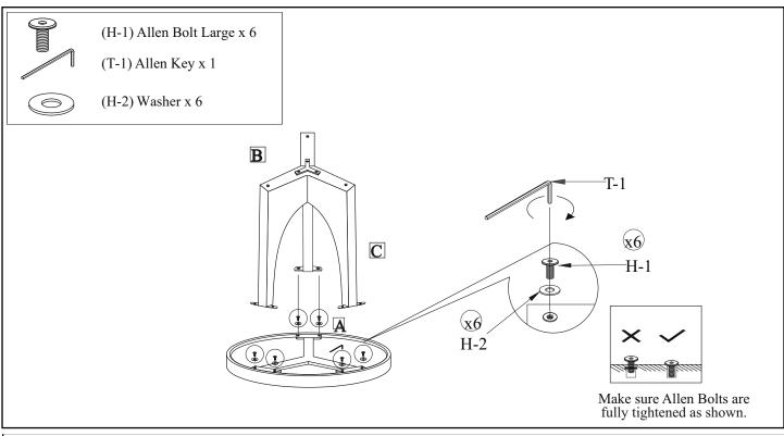
Place Wood Top (A) upside down onto a padded, non-marring surface. Position leg assembly onto the Wood Top (A) as shown, and align the holes. Secure connection with Allen Bolts Large (H-1) and Washers (H-2) using the provided Allen Key (T-1), stacking the hardware in the order as shown. Now fully tighten all hardware from this and all previous steps. DO NOT OVER TIGHTEN.
